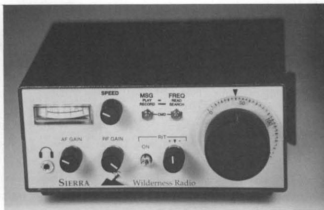
Front view of the completed Sierra. The meter and KC-1 controls are not part of the basic Sierra kit.
