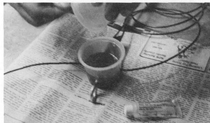
Photo 2—Pour resin into the mold; be sure to mix resin and hardener in a separate cup
