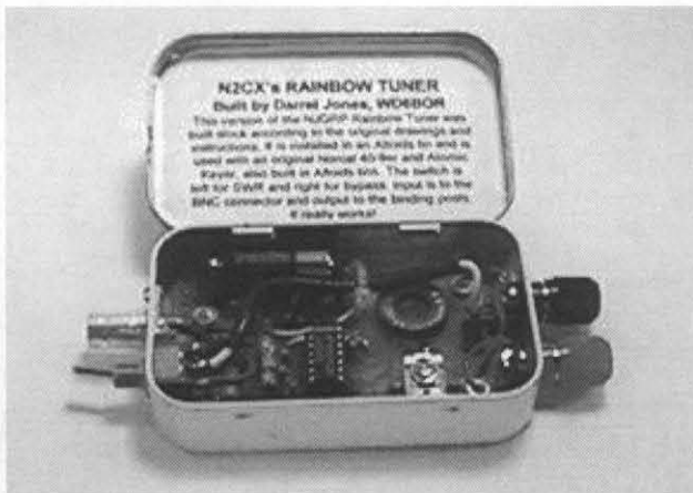
Rainbow Tuner built into an Altoids mint tin.
