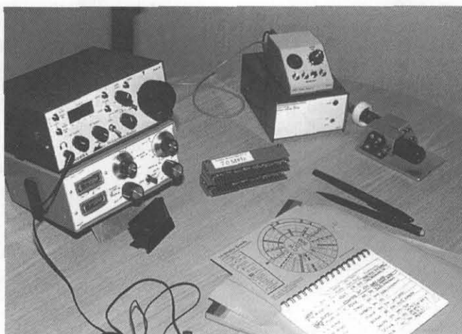
W6ZH/KH2 up and running. Pictured from upper left to right: Sierra (top), St. Louis Tuner (bottom), LCD clock (front) two Sierra band modules, power supply (minus switch), CMOS Super Keyer II (top) and Galbraith key paddle with remote keyer memory buttons.
