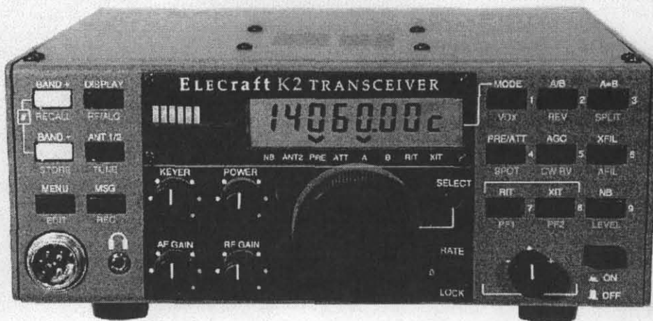
Prototype K2 Transceiver. The front panel buttons are multifunction; a short "tap" will activate the function indicated by the label above a button, press and hold will activate the function indicated by the label below a button. (Photo courtesy EleCraft)
