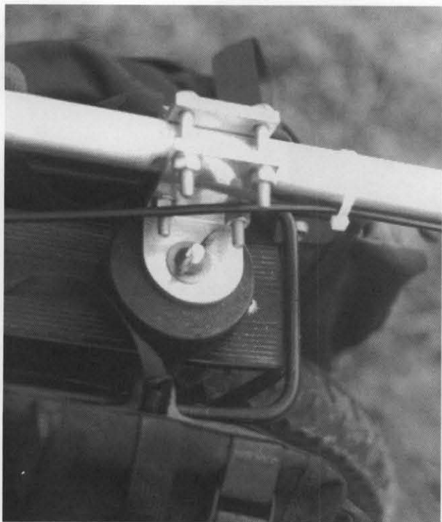
Pannier rack support for the antenna mounting system. Note the hockey puck!
