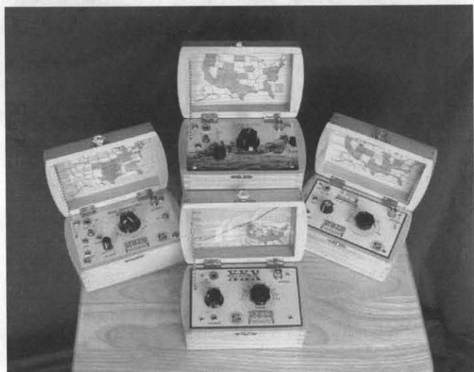
Figure 10. N5IB and WD5CMA family portrait. Clockwise from bottom: Herring Aide for 30 m, Small Wonder Labs DSW-40, Small Wonder Labs DSW-20 (USS Kidd version), NorCal 38 Special. Not pictured - Small Wonder Labs Green Mountain 30 (a bun in the oven).
