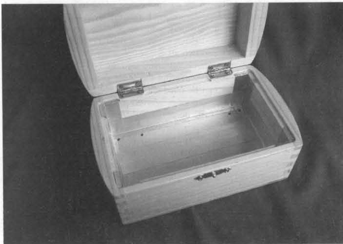
Figure 1. Note the rabbet around the rim of the box and the partial copper foil covering.
