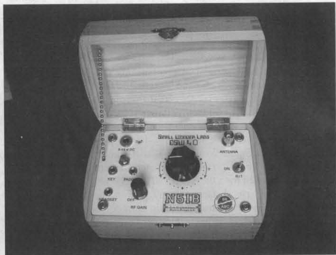
Figure 8. Finished panel installed. Note cup washers at each corner
