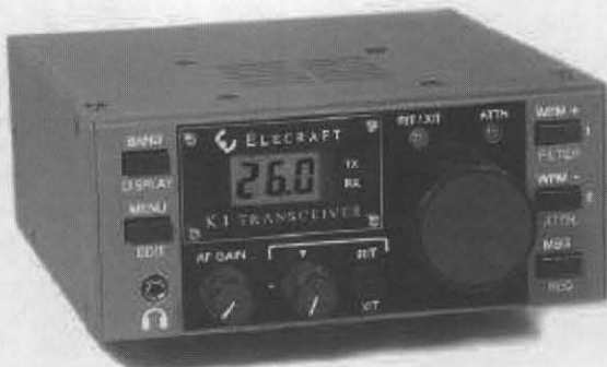
Figure 1: K1 Front Panel (Elecraft photo)
