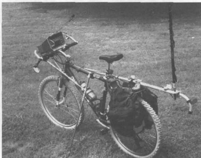
Figure 1. The K2/Gary Fisher Bicycle Mobile, complete with mini-paddles, boom microphone, and Outbacker Perth Antenna
