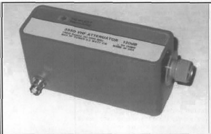
Figure 20—Hewlett Packard model 355D, 0-120 dB in 10 dB steps. (This particular unit is a relatively late unit; older ones have similar appearance although the color and style varied somewhat over the years.)
