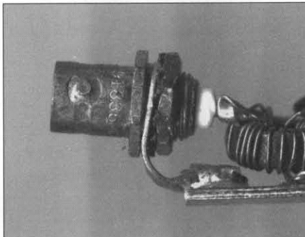
Figure 20—Closeup view of the solder lug used to hold the BNC. (Yes, this is one ratty connector on the outside but it still works great.)
