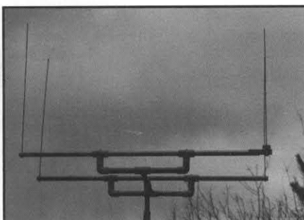
Figure 9 —A more complex PVC mounting frame for a 2-element 2-meter half-square beam.
