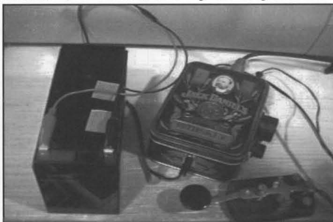
My Small Wonder Labs SW-20 QRP Kit mounted in an antique Jack Daniels Tin, along with 12v battery, straight key and earphone. A complete station.) Where else could you have so much fun for so little money?
