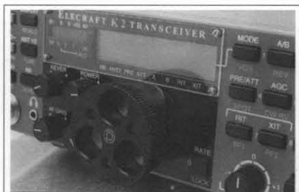
Figure 8—WW II vintage knob mounted on the K2 with homemade adapter
