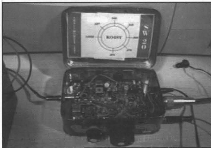
My Small Wonder Labs SW-20 QRP Kit mounted in an antique Jack Daniels Tin, along with 12v battery, straight key and earphone. A complete station.) Where else could you have so much fun for so little money?
