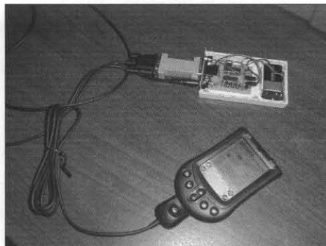
Prototype CW sender device with Palm m100 running prototype logging software.
