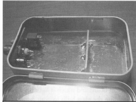
Figure 7—The doubler plate in place, and battery retainer wall.
