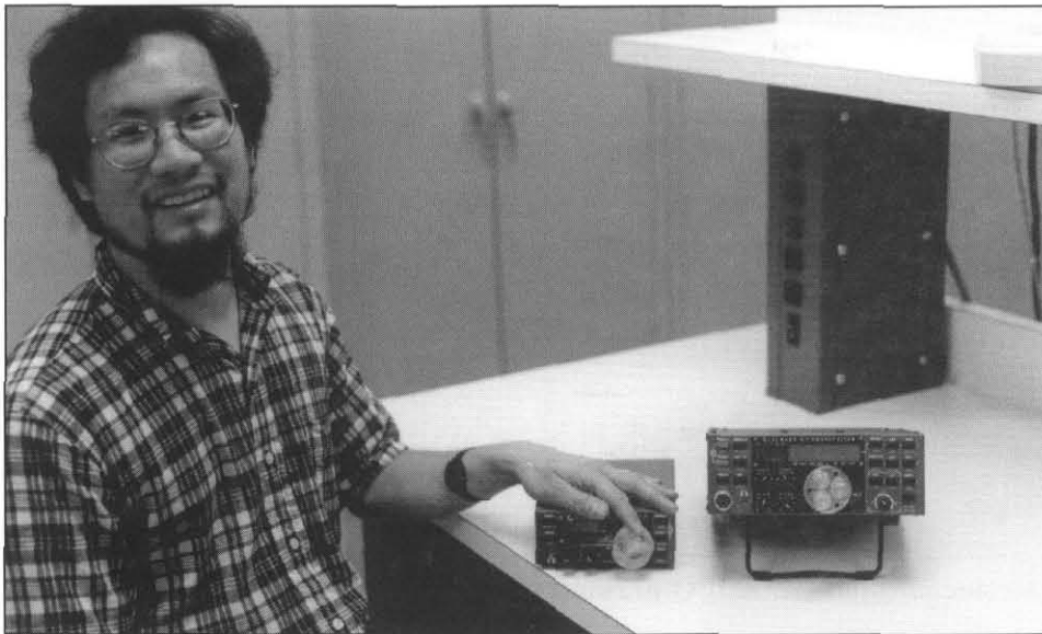
Figure 4—Zack Lau, W1VT, shows off homebrew knobs on his Elecraft K1 and K2 transceivers.
