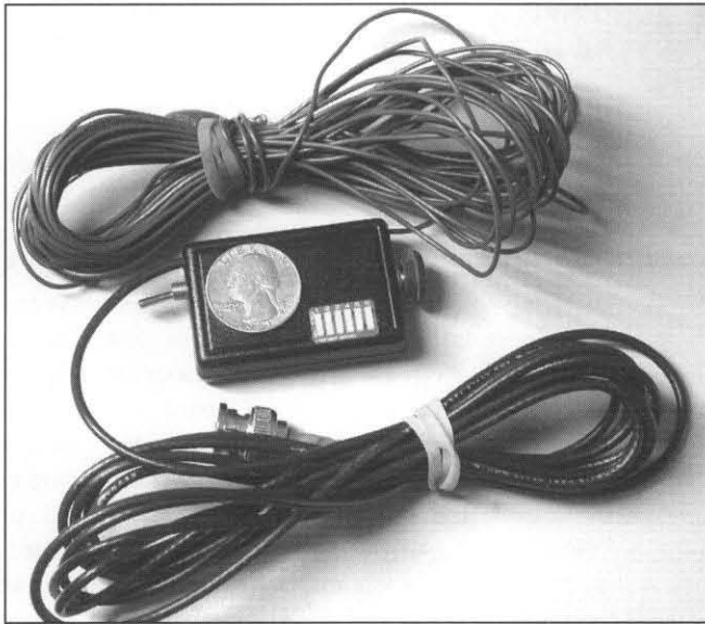
As this photo shows, the 20-meter end-fed antenna, tuner and SWR indicator makes a small package for portable operation.
