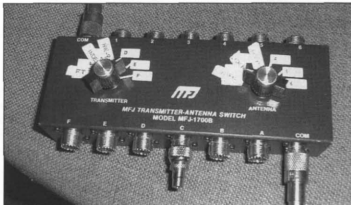
Figure 7—The MFJ antenna switch.
