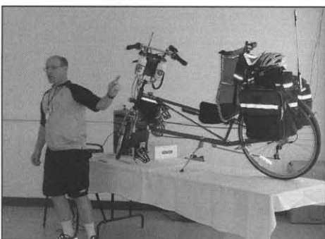
Anthony Norem, NØRJK, showing off his "bicycle mobile." The bike is equipped with an FT-817 transceiver, Z-11 Autotuner, battery pack and assorted antennas.
