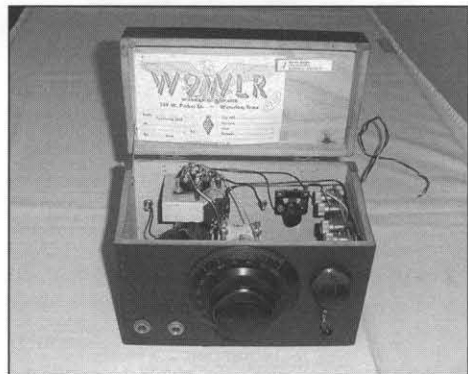
A close up of Warren's 1937 vintage single tube 5M transceiver. The rig is a super regenerative receiver in RX mode and an AM modulated self-excited oscillator in TX mode. Stability? We didn't ask...but he says that he made many contacts with it!
