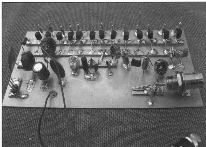
Figure 7—Strips of PCB material glued to the board provide connection buses for the bases and collectors.
