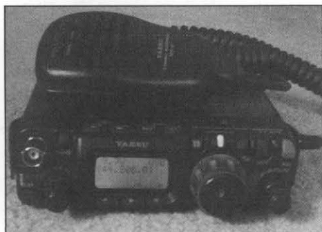
Figure 1—The Yaesu FT-817 QRP transceiver covers all modes on HF, 6 meters, 2 meters and 70 cm.
