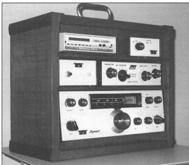
Build this complete portable shack with Ten-Tec Argonaut 509, power supply, antenna tuner, multi-mode controller and filter unit.
