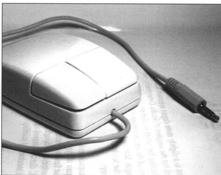
Figure 30—Modify an old mouse a bit, put a different connector on the cable, and it becomes a free set of paddles for your keyers.
