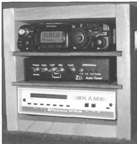
Figure 4—Completed portable shack for K8ZT's FT817, with a multimode TNC and LDG autotuner
