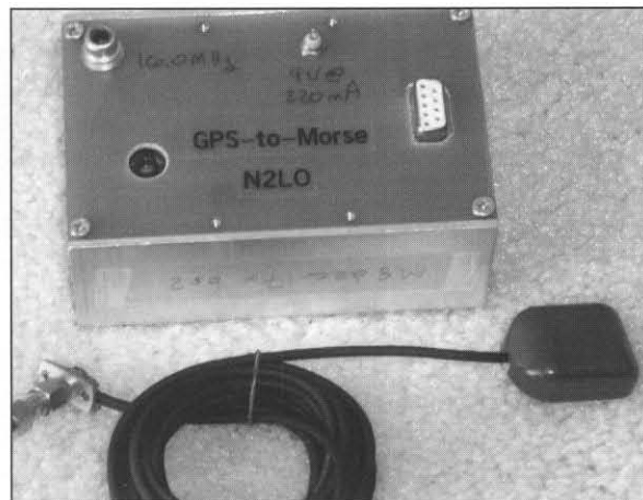
Figure 2—GPS-to-Morse box and antenna.
