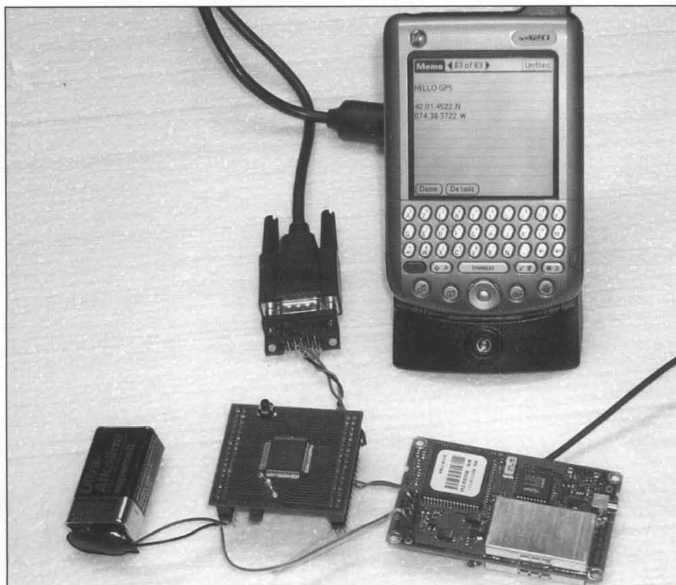
Figure 1—HC908 and DDS daughtercards controlled by a Palm PDA as a serial terminal for issuing commands and displaying messages.
