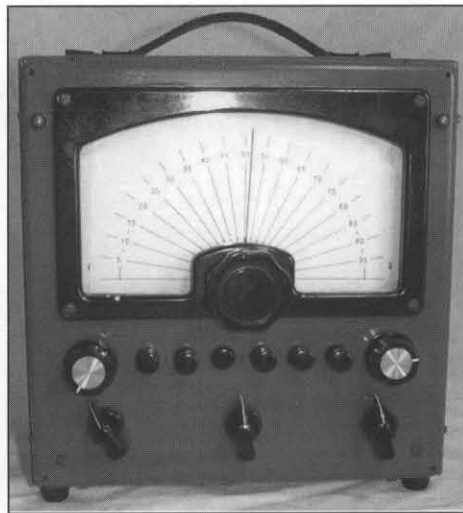
KG4CUY's homebrew 20M transceiver, built into a refurbished signal generator cabinet.
