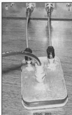
Figure 22—“Mint Tin” return loss bridge.
