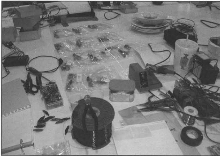
A key to a successful Building Day is the work area-set out materials at each workstation—a copy of the instructions, plus all other necessary components and materials.
