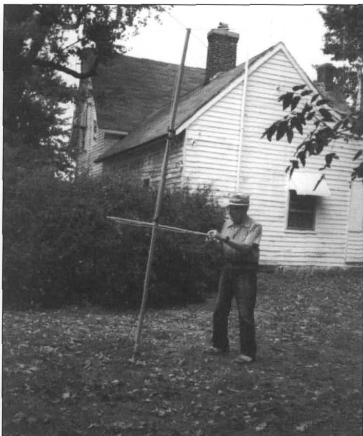
W9PNE adjusts the end-loading wires to tune his 20M short vertical dipole.
