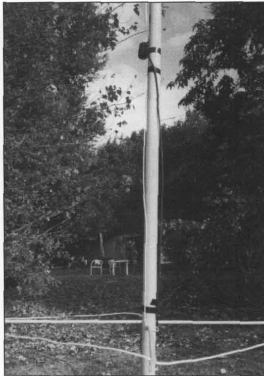
A close-up look at the construction of W9PNE's short vertical dipole. Note the spreader arms to hold the end-loading wires and the shunt (beta) matching coil across the feedpoint, wound on a 35 mm film canister.
