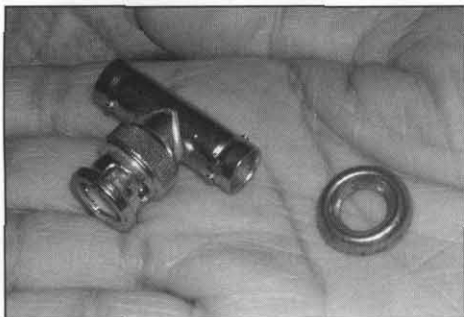
Figure 7—One of the chrome trim washers. Epoxy one of the black nylon washers to the knob to make a dimple for fingertip spinning.
