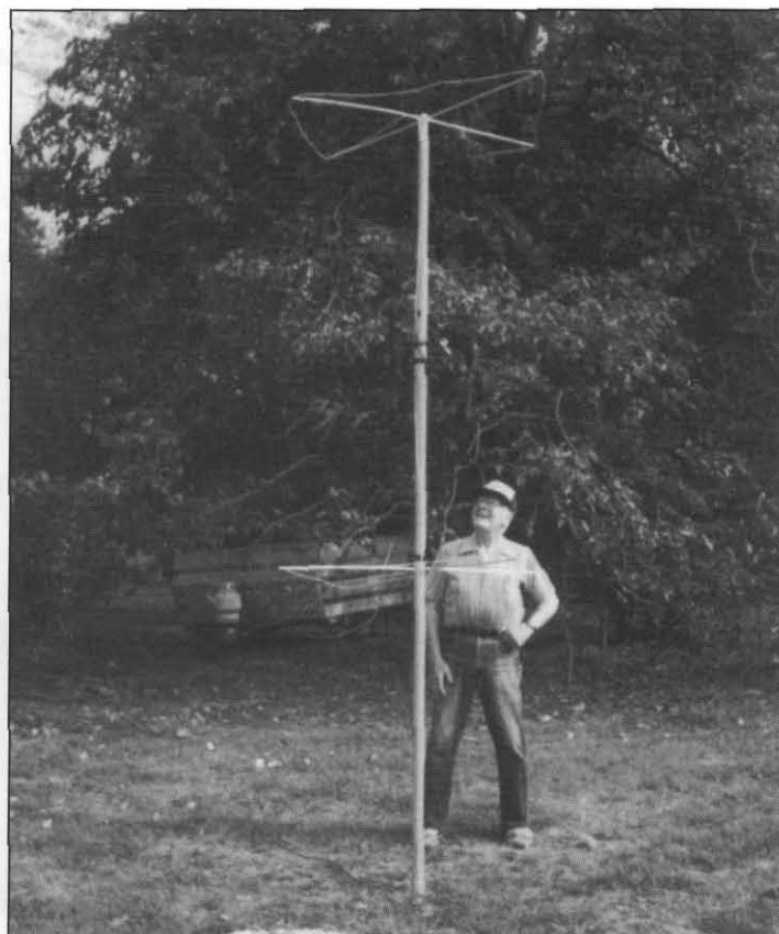
The finished antenna is held upright by slipping it over a rod-type electric fence post.
