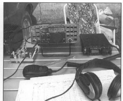
The UE3QRP/3 QRP station setup: K2 and FT-817. Operation included CW and PSK modes.
