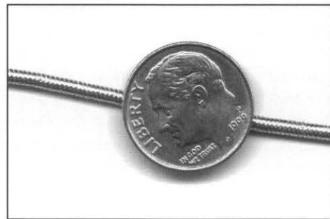
Figure 13—Some Belden 1671A cable, about the same size as RG-174 with the plastic jacket stripped off.
