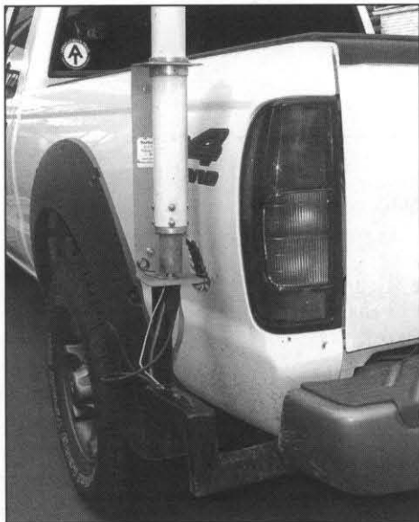
Photo 2—Close-up of the custom welded mounting bracket for the screwdriver antenna.
