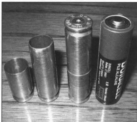
Figure 10—Left to right: .45 shell, cut down 30-06 shell, completed dummy cell, AA cell. Safety note: be sure the shells have been fired first.
