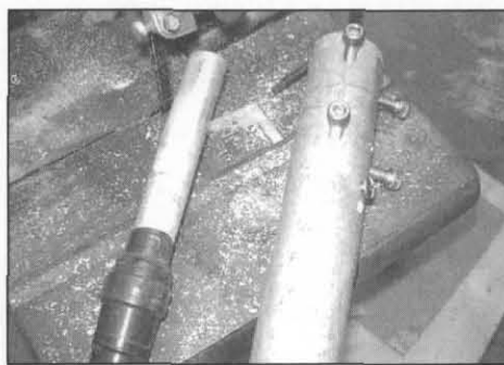
Photo 1—Mounting top pole onto scaffolding pole.
