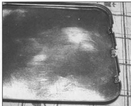
Figure 9—Cover of the AOL tin with notches cut in the side to accommodate the connectors and switch.
