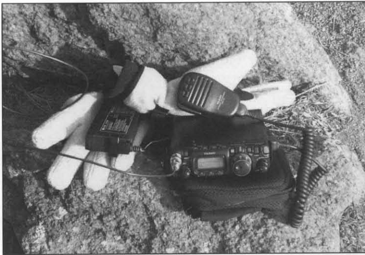
Photo 2 —The primary VHF rig for the January contest effort is the Yaesu FT-817.
