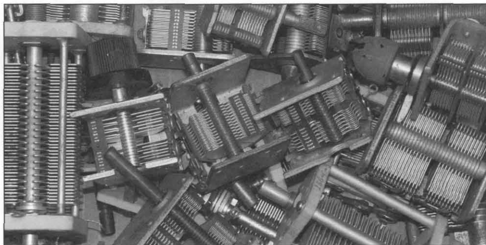
Figure 1—“What about that air variable?” Just about any capacitor in your junk box can be used to build a working VFO.
