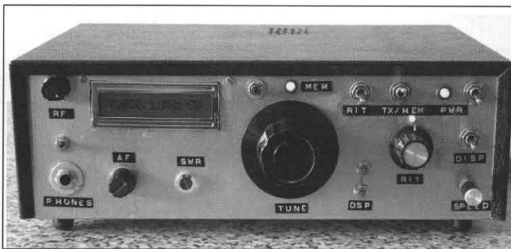
Figure 1—EI5EM's Bosca 40, a one-box 40M QRP station.
