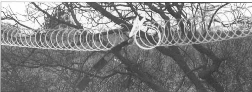
Photo 1—Darren, GW7HOC, has this "Slinky" 40 meter antenna.
