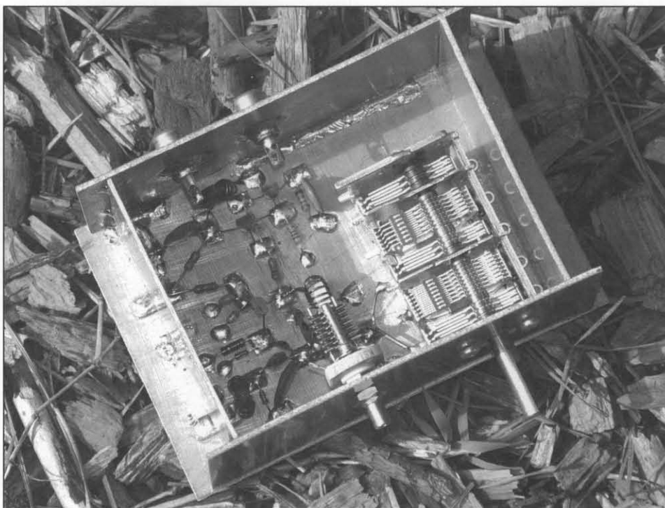
Figure 7—Completed 7 MHz VFO module; note Ocean State air variable used in this particular VFO; also note notches on left side for +12V (rear notch) and offset (front notch) pads.
