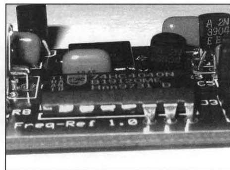
Figure 2—Close-up showing how pins are cut off the IC.
