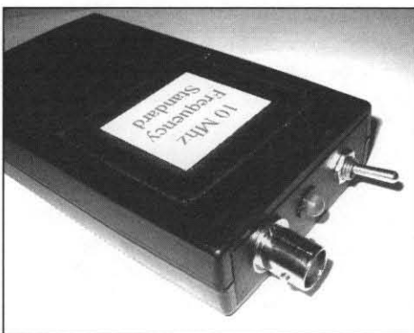
Figure 3—Finished frequency reference in a plastic case.
