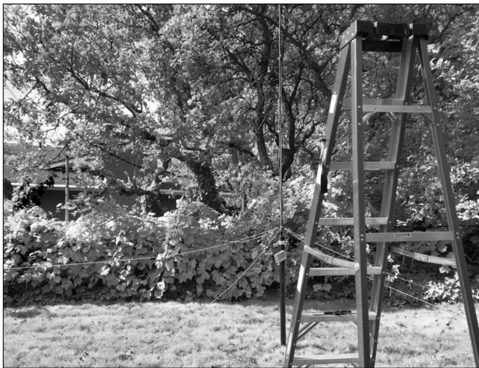
Figure 1—With a quarter scale model, even the top of the 40 meter element is accessible from an eight foot stepladder, provided one or two sections of the mast are collapsed.
