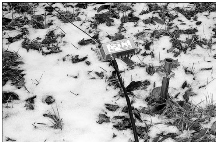
Figure 4—Photo of the feedpoint. At the other end, there is a 1000 Ω terminating resistor between the wire and ground.
