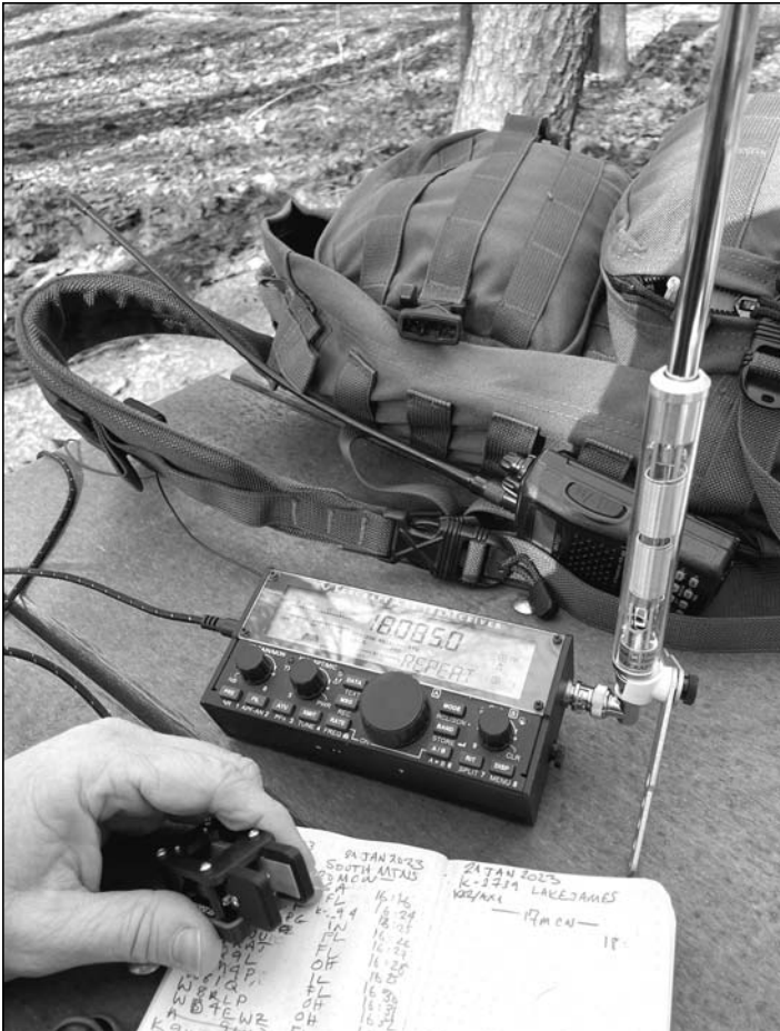
The Elecraft AX1 4 foot vertical is designed for portable operating; shown here with the KX2 transceiver.
