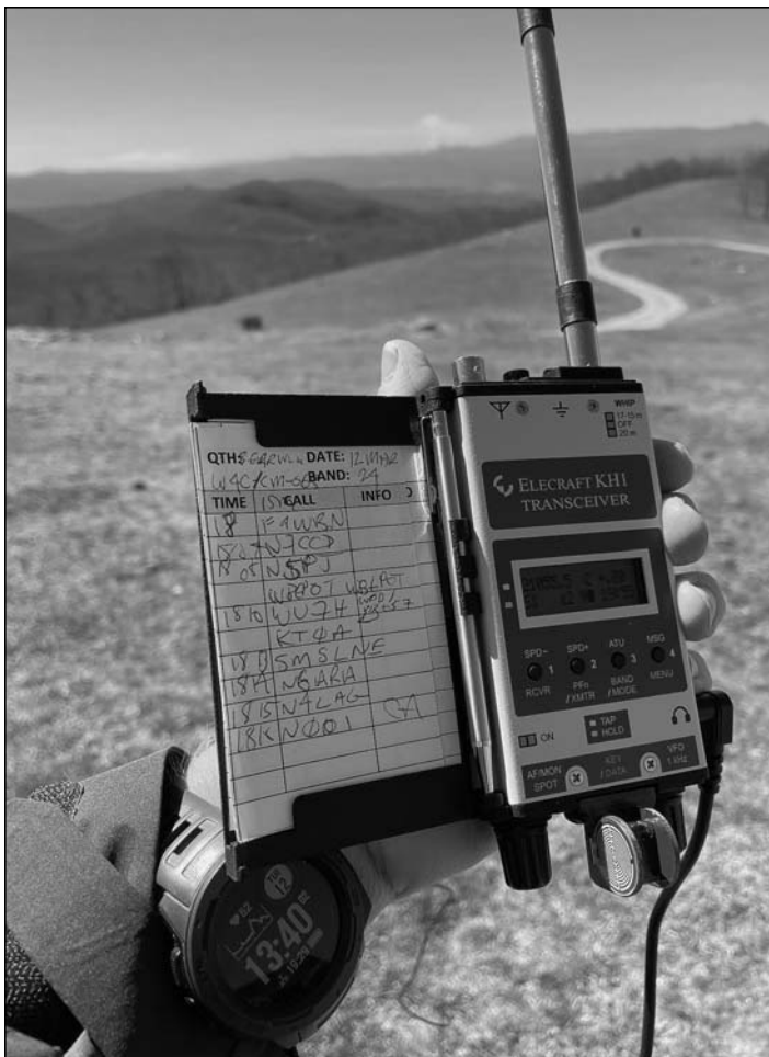
The new Elecraft KH1 Elecraft KH1 is ultra-portable, weighing less than one pound.
