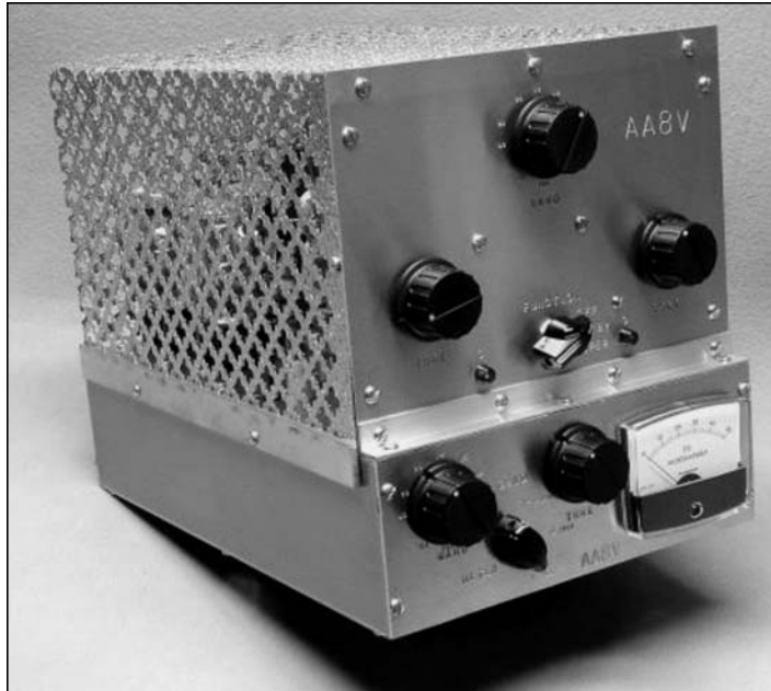
An example: 6146 linear amplifier.
