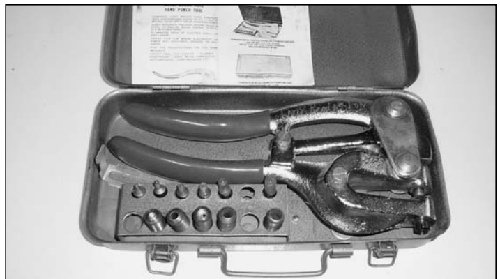
Photo 2—A copy of the Roper-Whitney hand punch. There is no identification of its manufacturer.
