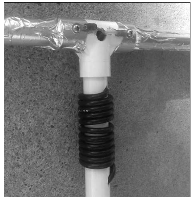
Detail of the coax connection to the driven element.
