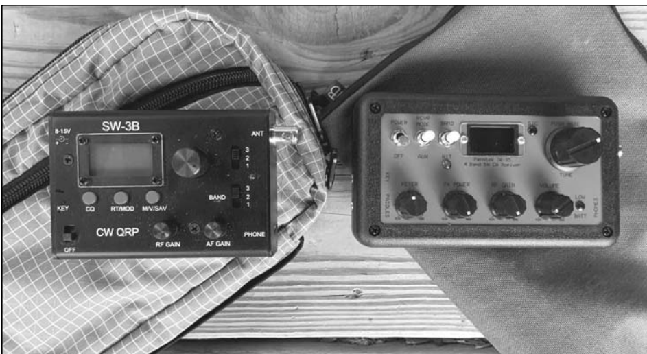
Two popular portable rigs—the Venus SW-3B and Penntek TR-35 (along with the padded carrying bags that I use).
