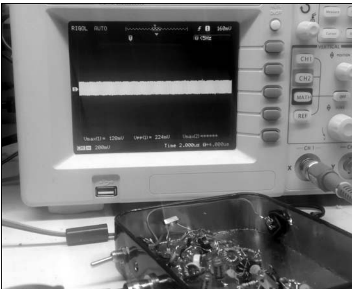
Output with one tone in operation.
