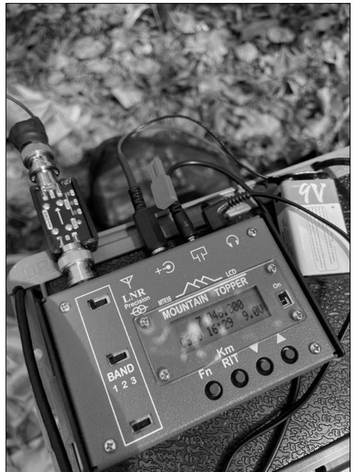
My MTR-3B, operating in the Rocky Mountains with only a Lilon 9V battery for power.
