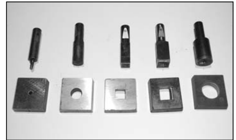
Photo 4—Some of the dies available for the Heinrich press. The company offers round and square dies up to 1/2". I used a grinder to put a flat on a 3/8" die for either a BNC or F connector. And I had a local tool-and-die shop make a 5/8" die for UHF or type N connectors.
