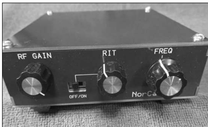
Figure 6 —A closeup of the NORCAL 40B front panel, Using PCB material makes neat labels.
