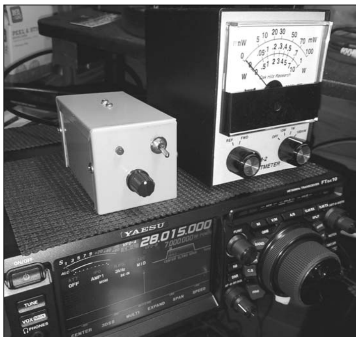
Here is the ALC power control box on top of the FTDX10.
