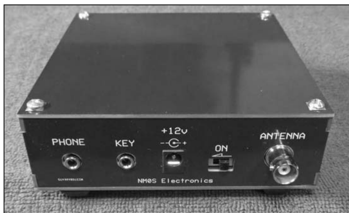
Figure 7 —The real panel includes connections for head-phones or speaker, a key, 12 VDC power input and RF
