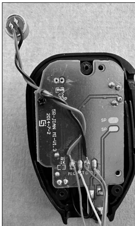
Figure 5—Connections inside the modified microphone.
