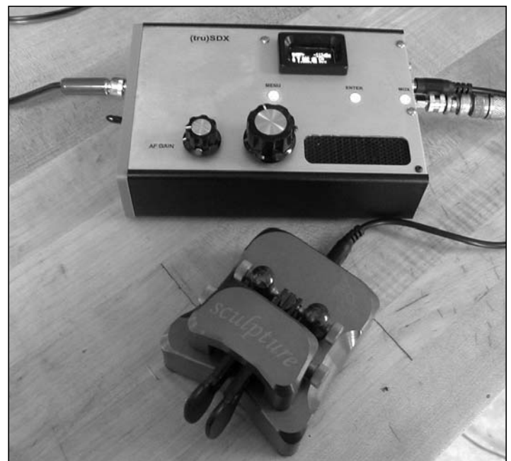
Figure 6—An overall view of the finished upgraded transceiver, ready to operate with a CW paddle. The new lighted switches are also visible.
