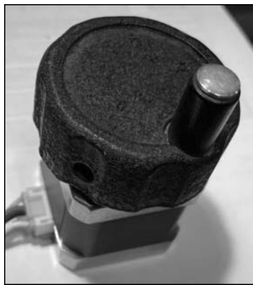
Figure 7— The 20:1 reduction gear and the tuning control knob are taken from a BC348 WWII military radio.
