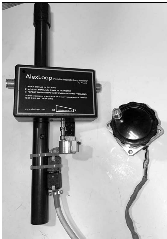
Figure 5—Here is the AlexLoop with the remote tuning system installed.
