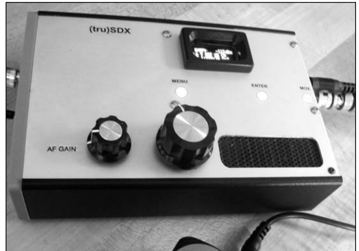
Figure 5—Front panel view of the upgraded unit.
