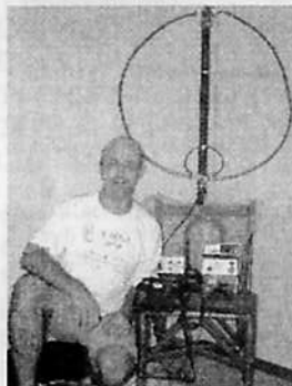
Juan with his magnetic loop antenna which he used as XE2/EA5XQ in Monterrey during 2002.
