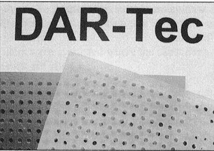
A company local to the G3RJV has begun to manufacture a range of Matrix Boards. DAR-Tec produce a plain 0.1" spaced matrix board (Perfboard) in two sizes and in translucent FR4 material. They also produce an interesting matrix board which is completely copper clad on one side. This is ideal for forming a ground-plane – remove the copper around the hole with a countersink drill for insulated entry or leave the copper in place for a ground connection.
