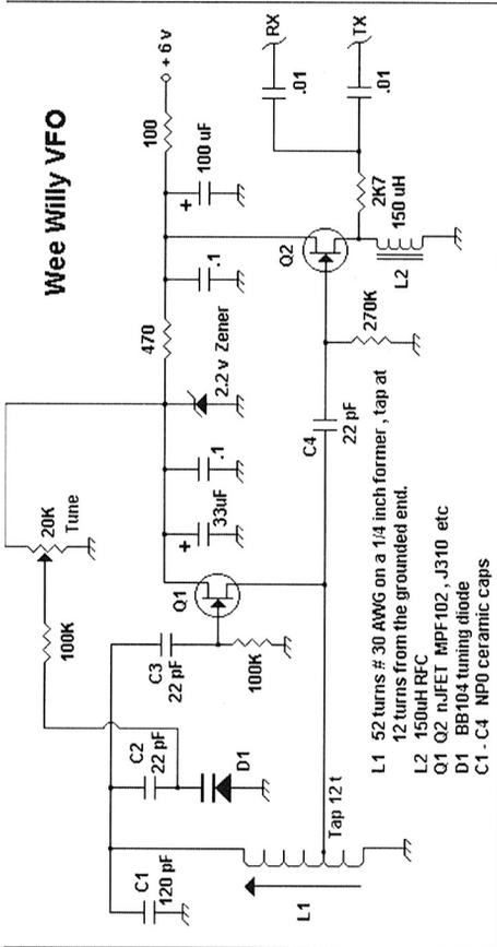
Try checking an old television to find suitable coil formers. It would probably be best to distribute the 120 pF C1 capacity among 3-4 capacitors to enhance stability. These caps should be NP0 ceramic for best results with frequency stability.
