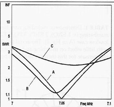
**Fig. 2** EZNEC<sup>TM</sup> VSWR curve minima relative to 52 ohms for the aerial in Fig. 1. (A) perfect ground, no losses:  $F=7.05\text{MHz}$ ,  $\text{SWR}=1$ ,  $Z=52$ . (B) Copper losses:  $F=7.044$ ,  $\text{SWR}=1.14$ ,  $Z=59$ . (C) Real (see text)  $F=7.062$ ,  $\text{SWR}=2.22$ ,  $Z=110$ .
