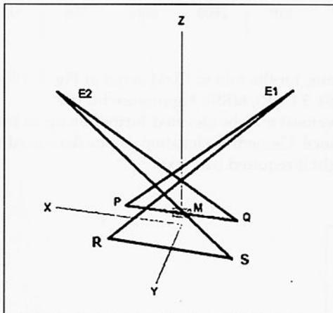
**Fig. 1** Revised folded IIDM aerial without the need for explicit ground connections. PQ contains the matching unit M (see SPRAT 121).  $C_m=48\text{pF}$  and RS is a non-grounded bridging wire. All dimensions are given in TABLE 1.
