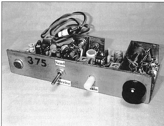
“Wee Willy”. is a double sideband transceiver. It has a low parts count and is easily built using non-etched PC board techniques. It has a homebrew case using copper clad PC board for the front and back panels and cardboard for the rest of the case. The set itself is in a case 1 1/4 by 2 1/4 by 5 1/2 inches. There is a separate container which holds a 6 volt rechargeable battery and
