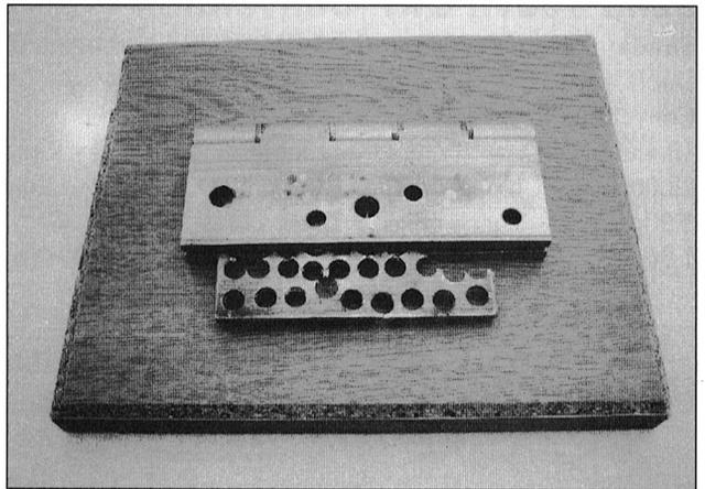
I drilled a hole in two flat metal bars and placed a piece of single sided PCB between and gave the punch a good hard bash it produced the desired effect, but it was damaging the back of the single sided board. I thought I would try to punch the islands out in double sided board, so I tried again, this time success, no damage to the islands.
