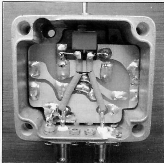
The SWR Bridge on a pcb and
