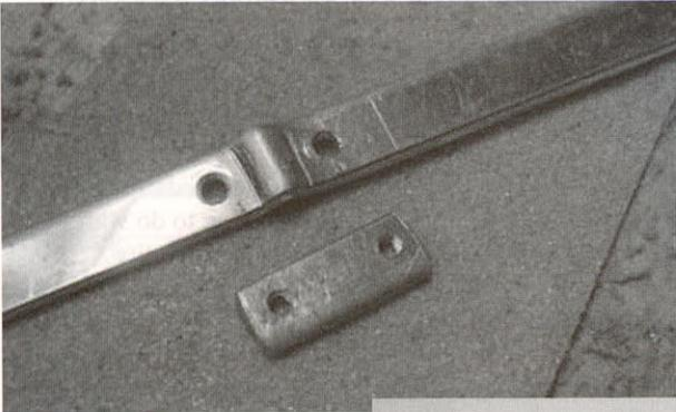
A small piece of brass is made for locking the key arm to the pivot.
