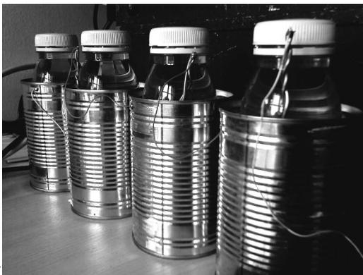
from ASDA supermarket). The water in the orange juice bottle makes it easier to wind the wire without the bottle compressing, and weighs it down in the can. The can is negative, and the copper wire positive. The Johnson's bottle keeps the wire perfectly close to the can but not touching, and also reduces the volume of bleach required: one 750ml bottle of bleach is very cheap and enough for four such cells, which produce well over 3V when connected in series.
