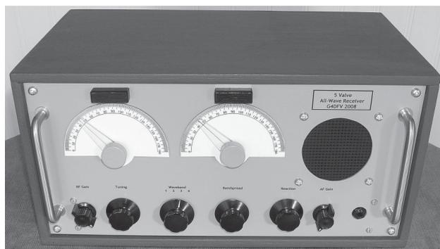
**G4DFV** has just completed a five valve TRF receiver that tunes LW, MW and two short-wave bands (see picture left). It is based on the receiver circuit of the WW2 'Paraset' with the addition of an untuned RF stage and an audio power stage. Duncan says reproduction of AM commercial broadcast stations is superb and CW and SSB on the amateur bands is ok.
