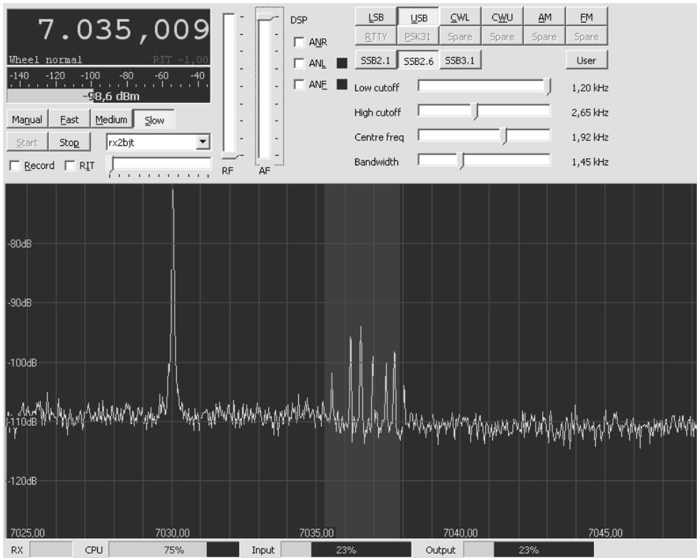
Figure 3: The MOKGK's program shows seven nice PSK31 signals near 7036 kHz. Use WINPSK to decode them.
