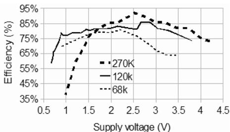
These graphs show the transmitter's power output and efficiency (RF power output as a proportion of overall circuit power consumption) into a 50-ohm resistive load, using different values for the 68k base bias resistor. Oscillation continues all the way down to 0.5V supply! Note that there is no filtering of harmonics and therefore this data is probably over-optimistic, so these graphs should be taken with a pinch of salt (not bleach).
