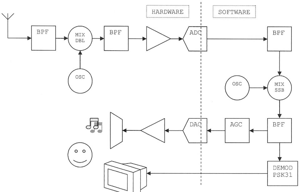
Figure 2: the signal path over hardware and software blocks
