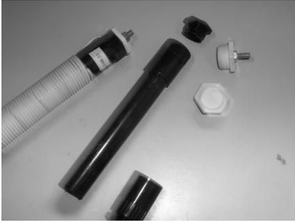
We are using 20mm conduit instead of the American PVC risers to make the loading coils there is a difference of 0.5mm in diameter. (Risers are 19.5mm) The ends are made up of 20mm adaptors and blank plugs both of PVC obtainable from electrical wholesalers. The blank plugs are drilled through their centres to take the set screws and nuts for attaching the rods of the antenna.
