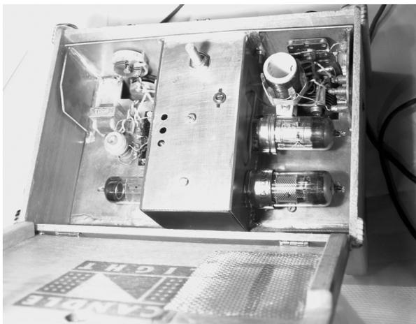
VFO controlled tuning of the entire band, only little warm-up drift (200 Hz/h)
