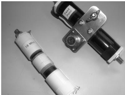
The feed point insulator at base of the antenna is again made from 20mm PVC (in fact I used a piece of 25mm to make it more robust but your 20mm will do ok) Instead of using the bolt through the conduit and aluminium strip to attach the counterpoise wires I fitted and extra screw and nut tightened to it and then a wing nut to attach said counterpoise wires. (See photo) I also used 2 of 4mm set screws and nuts to affix aluminium plate to conduit to stop tendency to swing round.
