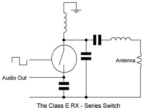
I shared this idea with Wes Hayward W7ZOI and he suggested I try using the MOSFET as a shunt switch - this works as well. The T/R switching and muting is a bit more complex to implement than the series switch version. Experimentation is needed...
