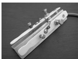
The basis of the paddle is a 105mm length of aluminium angle 20mm x 20mm x 2mm (mine came from B&Q). The paddles are made from any plastic and are 100mm x 10mm. I used sections cut from a shatter proof ruler that are 2.5mm thick. The flexibility of the paddles affects the way the paddle feels in use so you may need to experiment a little. The thickness of the material as well as the length impacts the “springiness”.
