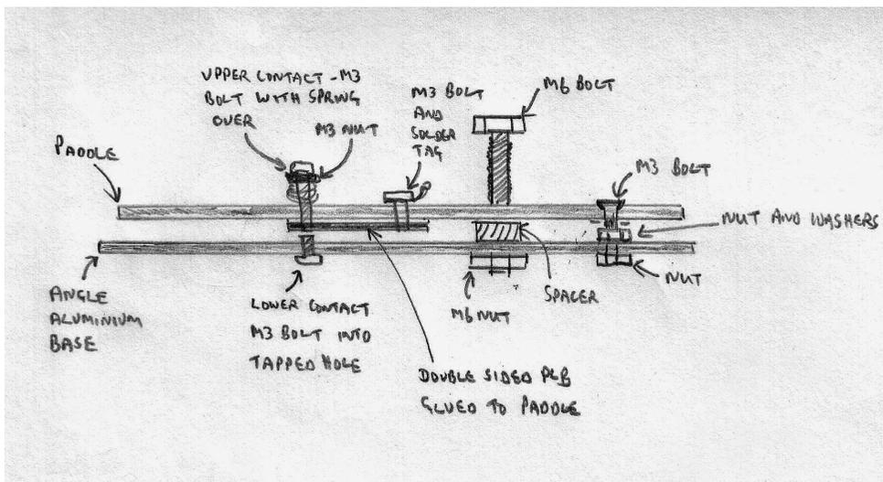
The paddles are fixed towards the back by two bolts. The foremost is larger and protrudes 15mm above the paddles. This provides an easy fixing for a length of button elastic (available from needlework and craft shops) which passes around your leg to hold the
