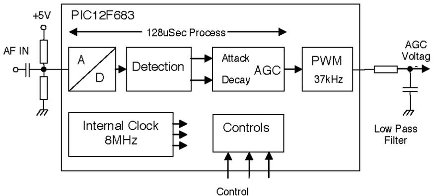
**Fig.1** AGC block diagram
