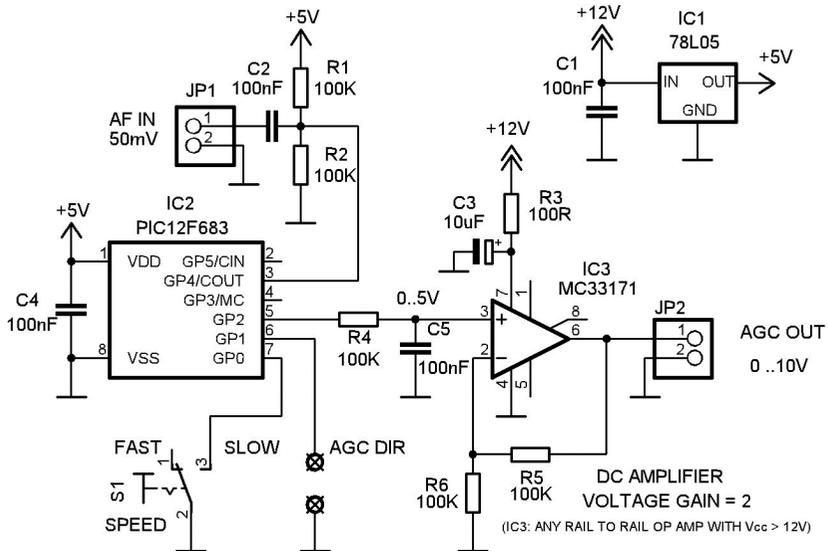
Fig.2 AGC system schematic
