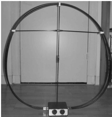
Loop with two capacitor tuner beneath
