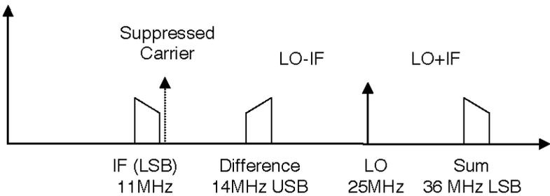
Fig. 1 *Frequency diagram for high side LO*
