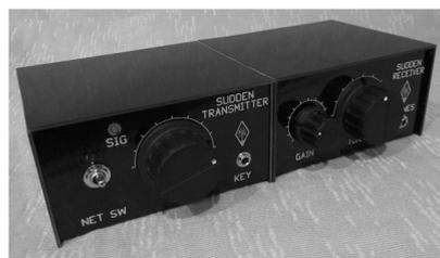
The transmitter output is 50 Ohms and will need an ATU unless the antenna presents the correct 50 Ohm load. The kit is now available for 40m and we are working on versions for 160m through 20m. The cost is £34 plus postage - £2 (UK), £3 (Eu) , or £4 (DX), and should be ordered from club sales – see the back page. You can download the full manual
