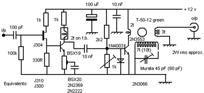
Notes: The overall gain is about 30 dB, so the o/p of a diode mixer for instance should give the full 2 w o/p. The 2N3553 needs heatsinking. Set the bias current for best linearity ( I<sub>c</sub> about 100 mA). Check there is no thermal runaway & fit larger heatsink if necessary. The 1N4003 should be in thermal contact with the o/p transistor.
