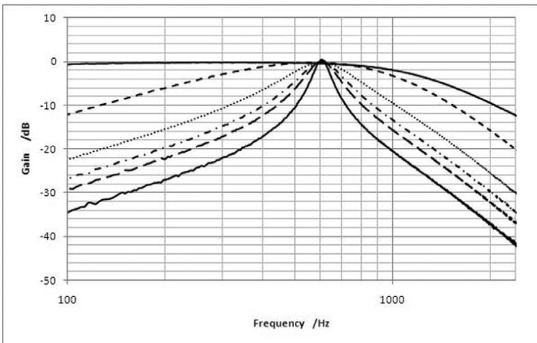
**Figure 3** Measured Voltage Gain of the CW Filter, showing action of R4 (R6 in mid-position)
