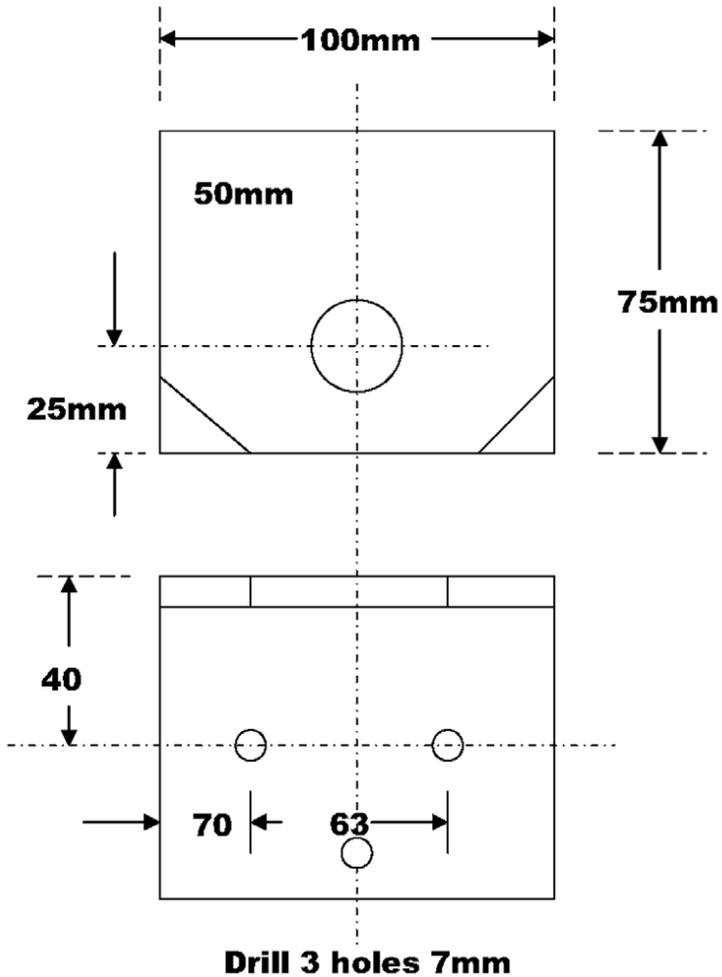
The third hole is for a 6mm nut and bolt to be fitted to pack out the base into the vertical. The metal work can be purchased from Metal Supermarket U.K. who has outlets around the U.K.
