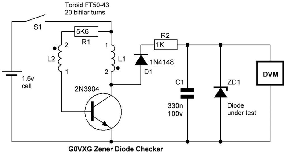
Having a quite a number of Zener diodes in my junk box, I thought it would be useful to know the values... Most constructors have a PSU that will go up to 12volts so it is relatively easy to check the values of low voltage diodes. However when it comes to checking voltages above 12 volts you finish up stringing a few batteries together to reach the Zener voltage and it all gets a bit of a mess!
