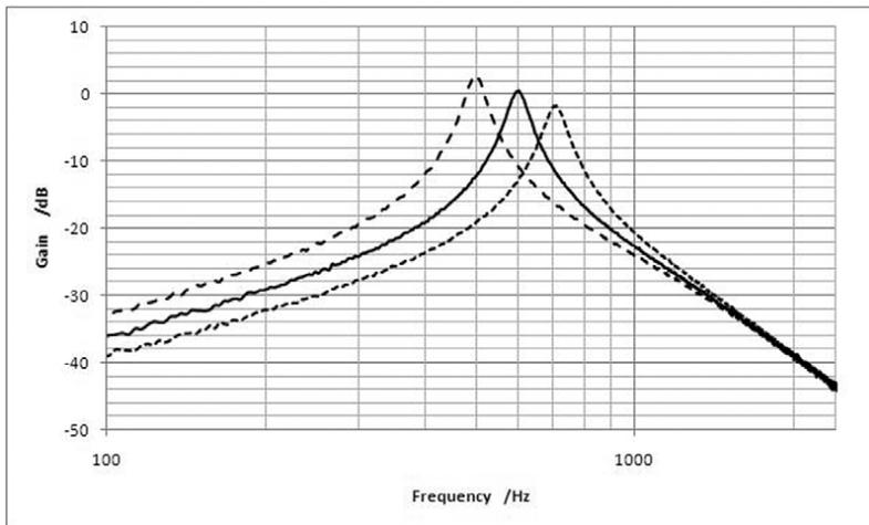
**Figure 4** Measured Voltage Gain of the CW Filter, showing action of R6 (R4 in max position)
