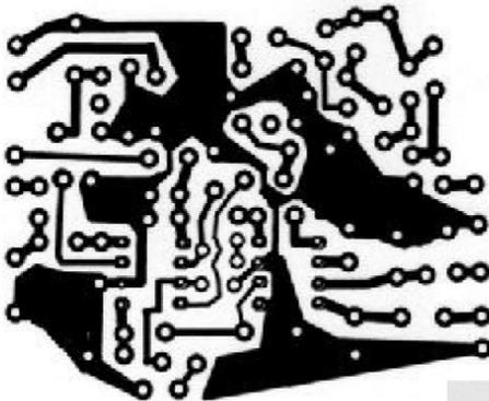
(Since the above was written – Phil ZL2NJ has drawn up a pc board. He etched it, dropped in the components and apparently it went “first time”. However, the aerial input coil and the interstage transformer used are more standard components, though you could still use the same as the original. The pc board and partial overlay are shown.)
