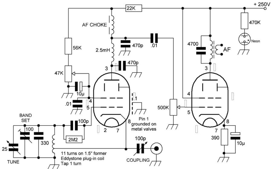
I used a plug in coil with the option of trying higher bands so if you want 40m or 30m you will need to juggle the turns and tank capacity. That whopping great 330 pfd across the tank along with the trimmer and low value tuning capacitor give good bandsread, (mine covers the first 80 KHz of 80m - what more do you want?), and there is little pulling of the received frequency by the attenuator trimmer in the cathode tap circuit.
