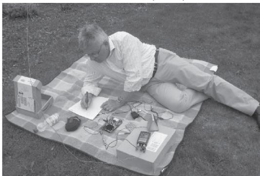
idea in *SPRAT* 144. The BS170 used as an electronic switch, offers high efficiency. It is excellent for QRP using eight Mignon alkali cells. The receiver draws 17mA and the transmitter 230mA. The first QSO with it was with DJ7JE at 559!". WA0ITP reports, "OzarkCon was a rousing success this year. It was held on 8/9 April in Branson, MO and set an all time record for attendance". Terry also reports that *QRPspots.com* has passed the 100,000 hit mark with 118,461 on 6 April.
