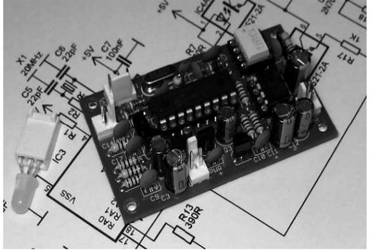
website for more information and example installations. The X-Lock kit comprises double sided, high quality silk screened PCB, pre-programmed processor, all components, connectors, IC sockets and a comprehensive step by step instruction manual. Just add 12v and a VFO!
