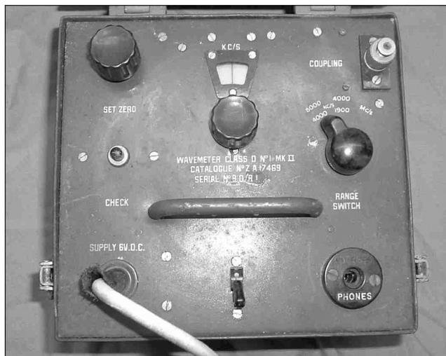
Have you ever thought to look at one of these in a different light? You might after reading this. The Class D wave meter was designed to measure and generate frequencies between roughly 1.5 to 9Mc (to 1kcs) and contains a variable oscillator on roughly 3.5 or 6.5Mc/s as well a crystal controlled one on 100 or 1000Kcs. It has a built in 6v vibrator power supply. I take my hat off to the designer, as it is a very clever piece of apparatus indeed.
