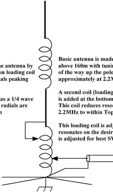
Tune the variable capacitor for highest RF field a small distance away from the antenna
