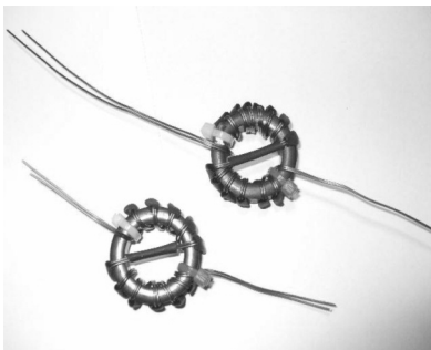
Figure 4. The twin FT114-43 cores wound with 14 turns
