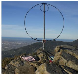
This is the DXLOOP used by **IK5XCT** to make his 5W QSO using his FT-817 with **LU6EF** on 17m in the Winter Sports. The loop is 47¼ inches diameter in Cellflex SFC12-50 and covers 40-15m. Stefano says it has 82% efficiency on 17m compared with a full-size dipole half-wavelength high. More pictures and info about it on his website at <<http://www.qsl.net/ik5xct>>.
