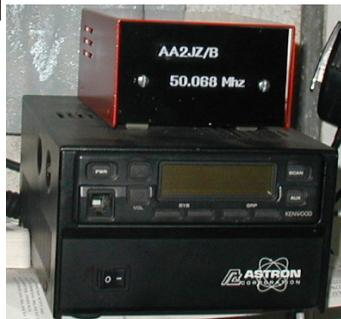
A 6m beacon on 50068kHz PIC16F628 controller, about 1W out to a vertical at 35ft.
