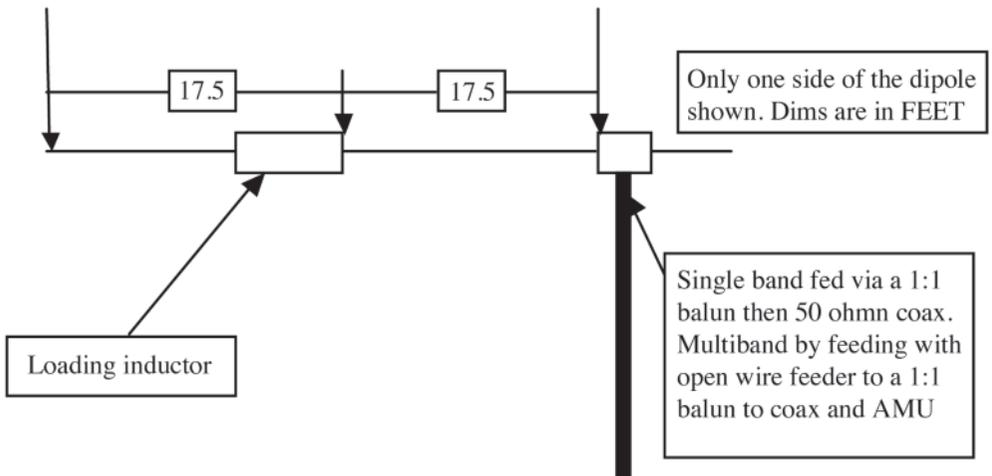
This is a simple short aerial for 3.7 Mhz. The idea came from the short GM4JMU dipole I used on 40m successfully in the past and I wondered about a short 80m dipole. There is a great web site for calculating the details of a short aerial at:
