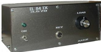
A Tube (valve) type transmitter for 3579kHz about 4W output.
