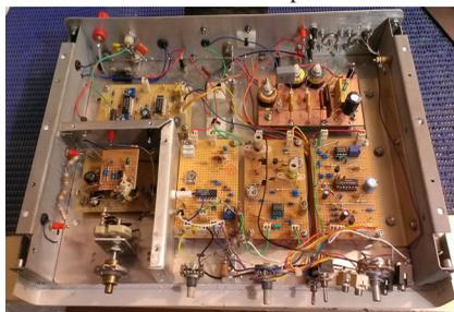
bit shabby. It was a **G4JXX** design and used four 555 timers; a nice simple circuit to understand and fault find. The photo right shows a new duplicate unit he has built in an old PC printer switch box. Chris says it works equally as well but looks a lot better!
