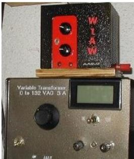
An 80m Reflex RX (above) and a variable voltage transformer with digital display, showing input AC voltage and variable output voltage.
