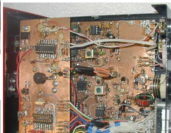
Interior of the 40m CW TCVR, all Manhattan Style construction, mostly salvaged parts. The case is a re-used AB Switch.
