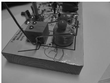
Above: The Mousetrap Receiver showing the “SMT” construction using drawing pins
