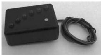
It is a very simple looking device – 34 x 49 x 20mm box with 6 LEDs (3 colours – 2 each of red, orange & green), and a single button that operates it. It is intended to monitor the voltage on rechargeable batteries, but it also covers a PP3 and a standard 13.8v mains supply.
