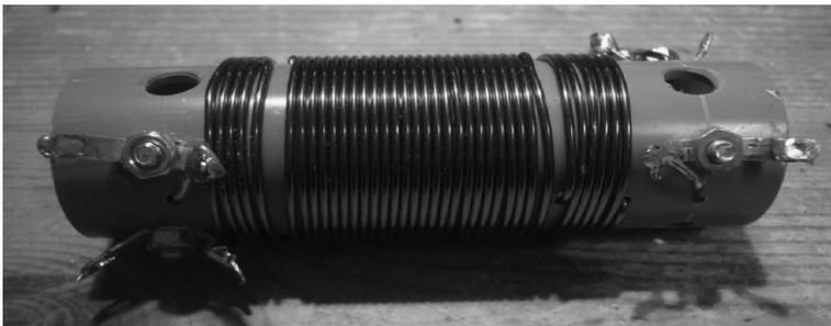
A solid construction is important for a good frequency stability of the RF frontend. Use wires with at least 1mm diameter and keep all connections short. The antenna coil (L1) has 5 turns, the tuning coil (L1 and L2) in total 31 turn with a tap a 6 turn from the end that is connected to ground. You can fix the windings with some glue to improve mechanical stability.
