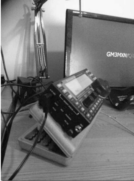
I was unhappy about the KX3 sliding on the bench supported on peg legs, and I noticed that I could purchase from the States a stand which is a bent metal support. Not having heavy gauge metal to make one, and no workshop, I thought about what I could use. I came up with what is shown here; costing nothing. I used an old socket set box. I cut two slots for the peg legs which keeps it from sliding right or left.
