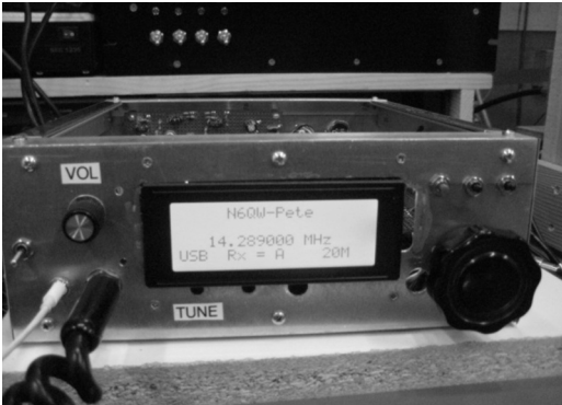
Figure 3 20m SSB Transceiver with Single DDS VFO
