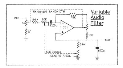
This simple circuit, very suitable for use with a direct conversion receiver, uses a 741 operational amplifier I.C. although a 709 could be used with slightly inferior results.
