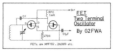
This circuit is basically an equivalent of a twin triode cathode coupled oscillator. By merely changing the tank circuit constants, output over a very wide frequency wide can be obtained - from far less than 1MHz into the VHF region. 30pF is a good compromise for the feedback capacitor Cf.
