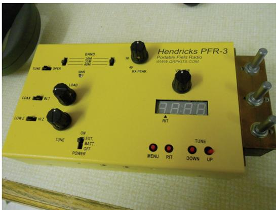
Well first of all, my favourite band was 40 and I do like to listen to SSB as well when portable. But the I.F. and Audio bandwidth is tailored for a 300HZ bandwidth specifically for CW reception. One "Field Friendly Radio" I have always fancied is the KX1 and so as the two circuits are very similar I decided to modify the PFR3 RX in line with the KX1.
