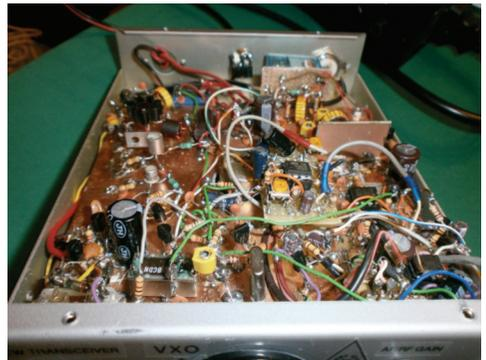
The audio filter is a OK1CDJ 2012 project. I found it as kit, sold on Ebay and made using SMD components. I built it with normal size components. It works fine and finally I have good reception “stand alone”, without help by Datong FL-3 audio filter.
