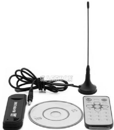
Note the MCX antenna connector; this is desirable as it provides better loss figures at the higher frequencies, although it is likely that you will change the antenna socket if you decide to put it in a metal box.
