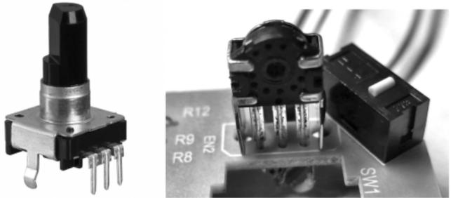
I simply connected the new rotary encoder across the contacts of the mouse wheel encoder and plugged the mouse into a spare USB socket on the PC. You can have two computer mice active at the same time on Windows PC’s.
