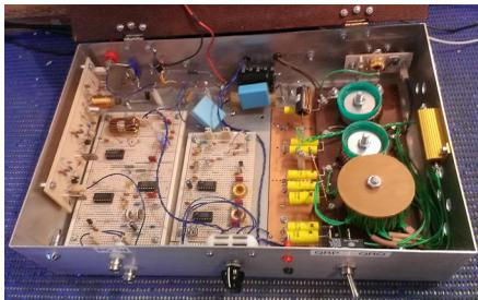
**G3XIZ** made a LF WSPR TX (above left) that is now fully operational and worked virtually straight away. It uses an up-converter requiring a stable 544kHz input which is generated from mixing two crystal oscillators. The PA uses a pair of IRF510 FETs in push-pull and the output power is adjusted using an old 'variac' auto-transformer on the unregulated DC supply. Chris was surprised that with only 5W of RF his signals were being picked up by **PA7EY** at a distance of 216 miles.
