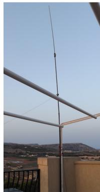
The picture above shows the balcony shack: FT-817, Bulldog mini-key, LDG Z-817 (in case the Buddistick didn't tune!), DYZ-8x7c speech compressor and Fujitsu M532 Android tablet for logging. The antenna picture shows the Buddistick on a ten feet telescopic mast bungi-cord fixed to the apartment railing.
