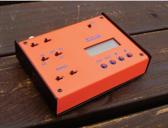
KD1JV's kit for 2015 was the fourth in the MTR series, called the MTR-5B. The rig now includes operation on five bands, a backlit four line LCD and optional rotary encoder.
