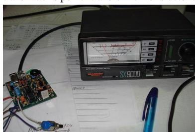
Left is the RockMite-20 DC TCVR that **YU7EO** bought at Friedrichshafen in 2015 and has working well producing about 400mW on 20m. Kare says the RX is quiet and sensitive, has two TX frequencies with one crystal, side-tone and el-key and in one word, is fantastic! In a day of testing it with a windom antenna in below average conditions, he made two-way QRP QSOs with **UR7VT** (2W) and **PA3DEU** (5W).
