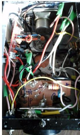
stage VFO fed into a BC108 and VN10 PA stage to give 500mW all
