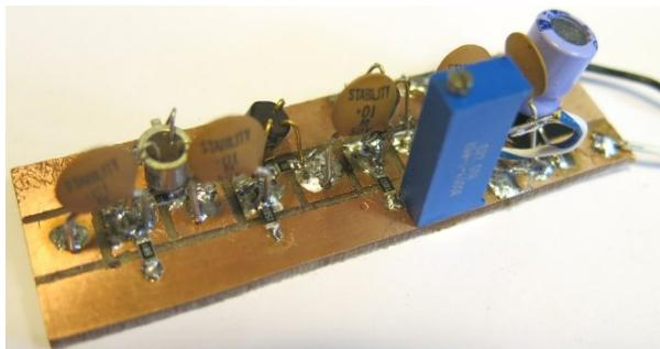
**G4WIF** has been doing quite a bit of constructing this year using the 'toner transfer' method of making PCBs, that has been very successful - as has making a board in five minutes using a quick milling method. This is Tony's **NOSS** zener noise generator; he says, "As you can see, the pads are cut pretty straight and work for both conventional and surface mount components, more detail on the two methods at <[www.fishpool.org.uk](http://www.fishpool.org.uk)>.
