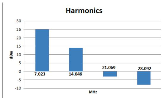
Reception is very broad (plus it also receives on the harmonics of the VXO). Sensitivity is hard to measure, but about 100uV. I am about 12 km from a cluster of AM broadcast transmitters in the 10 to 50kW range but there was no AM broadcast breakthrough as some have reported. On the other hand, a nearby AM transmission, even at low output, will break through – one of the well-known issues with the 386.
