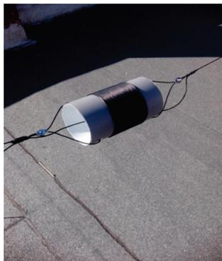
*The balun construction next the loading coils for the dipole.*
