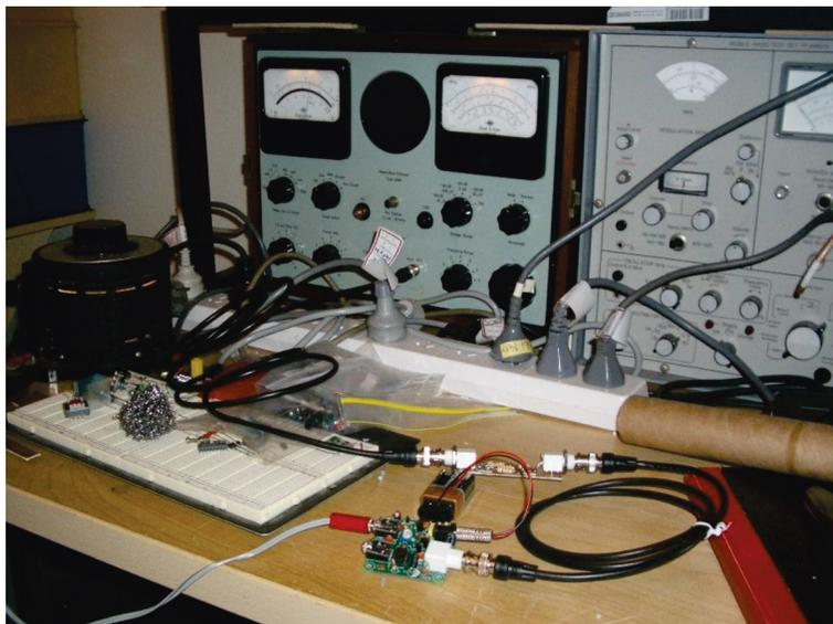
With a 12V battery, transmission power is 500mW, with a 9V battery, 300mW. Disturbingly, there is a 0.25mW output on receive because the VXO runs continuously.
