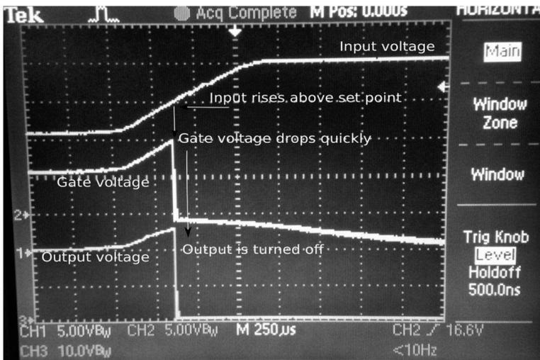
The screenshot above is an oscilloscope trace to show how the device responds to an input voltage over the threshold. At that trigger point the gate of the FET is taken low isolating the downstream equipment from the supply. When the overvoltage condition is removed there is a short startup delay before the supply is reconnected to the equipment.
