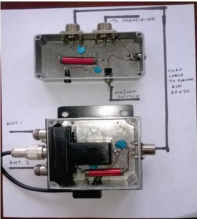
The project is in two parts, 1. Control box shack end, 2. Remote Relay box. The circuit is straight forward the only real decision is the choice of relay. For qrp good quality 12v car relays could be used, However I had acquired an aircraft antenna relay from some distant rally. So the choice of relay will
