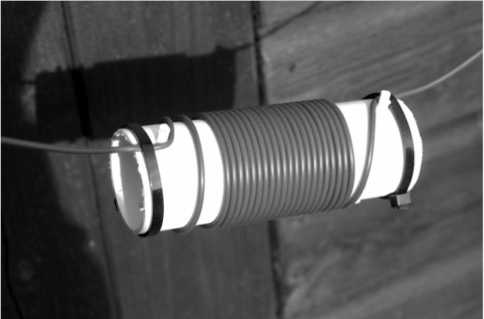
The antenna is constructed using SOTA-Beam green antenna wire (about 2.2mm diameter, PVC covered <http://www.sotabeams.co.uk/antenna-wire-lightweight-100m/>). Two 10.5 meter lengths were cut and terminated at a dipole centre insulator. I used a 1:1 balun but this is not essential.
