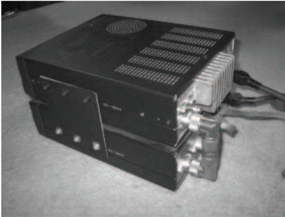
The mounting holes in the  $\frac{3}{32} \times 3\frac{1}{2} \times 4$ -inch aluminium plates were laid out to match the mounting holes on both the transceiver and tuner with the TS-50 sitting unsupported atop the tuner. The plates were secured with the metric bolts that came with the radio and mounting bracket.
