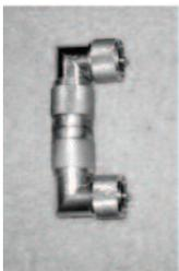
The  $\frac{1}{8}$ " tube was fitted onto the center pin of one 90° connector, then the section of copper pipe inserted into the threaded part of that connector. The other connector was then connected to the tube and pipe extending from the first connector. Finally, the copper pipe was carefully sweat-soldered to the two connector-threaded shells.
