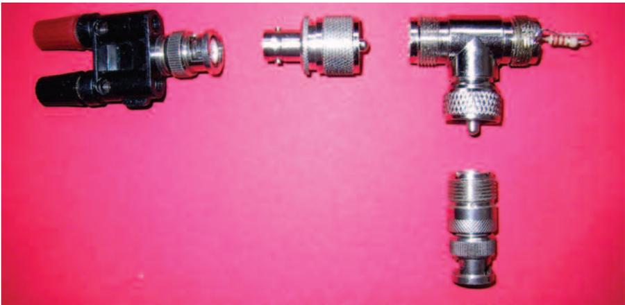
A little research told me that resistors between 1K and 10K would make a suitable drain resistor without affecting receive or transmit modes. I thought that I could install the resistor outboard of the radio and not have to find room in the innards.
