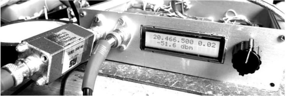
This is a 10MHz low pass filter, so the attenuation is shown as high – just as you would expect at 20 MHz.
