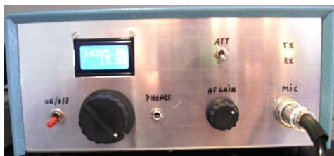
**PA3GNZ** writes "After a few years of building, I am not so active with home-brew, but my Iler20 project is ready (left). It produce 3.5W and I built in the DDS, so I receive the whole 20m band. In the case is a speaker to listen all the time on headphone, and on the back is a possibility to use the rig with 220V or 12V". Gose has used the rig for a few weeks and made SSB QSOs with **9H1FL/P**, **OE8NDR**, **SV9GPV** and longest distance
