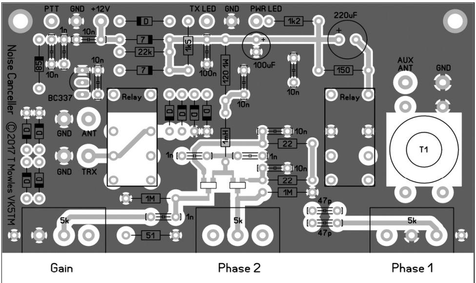
The diodes marked "D" are 1N4148's, "7" - 1N4007's and "85" - BAT85.
