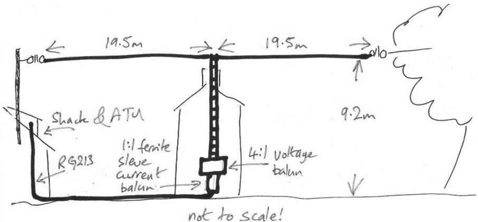
This looked ideal; it is a little shorter than the G5RV, but needs about two metres more height - depending upon the impedance of the ladder line. Unfortunately I doubt the present centre pole mounting arrangement could support an extra two metres, and the house is in a conservation area - and I don't want to push my luck!
