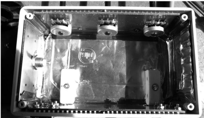
In the corners you might be able to see adhesive copper gardening "slug tape" to complete the screening. This is thick enough to solder to and is probably more effective used in the shack than when protecting my strawberries.
