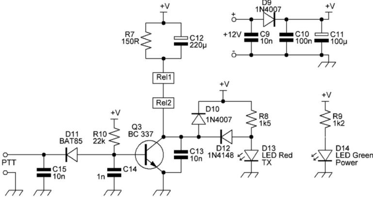
Fig 2 - Power supply and PTT section
