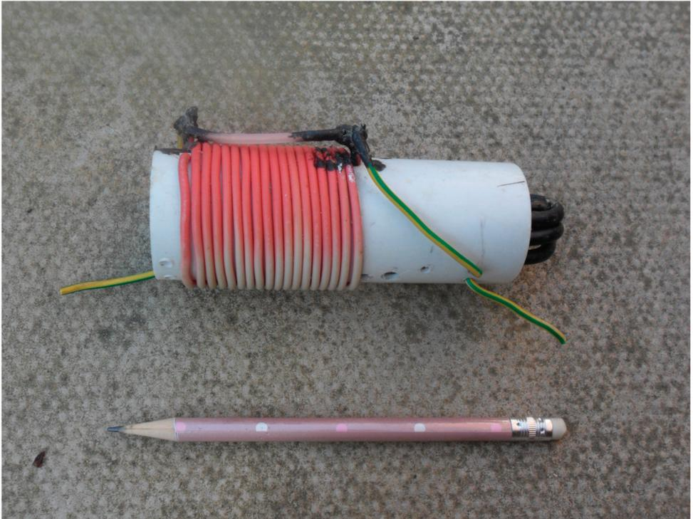
My red wire faded due to sunlight exposure over a 2 year service period. The black blobs are "liquid electrical tape" (ref 2) I had in stock and used for waterproofing the joints/ends etc. The coax is inside the tube and is just visible on the right.
