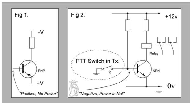
When Terry VK5TM sent me a prototype board for his noise canceller I did not have the BC337 transistor that he specified. We shouldn’t always get hung up about not using the exact component stipulated in an article – certainly not if it is a transistor used as a switch. As long as (in this case) it is NPN and it doesn’t get hot, it will probably work – eventually! My substitution didn’t quite – (more later).
