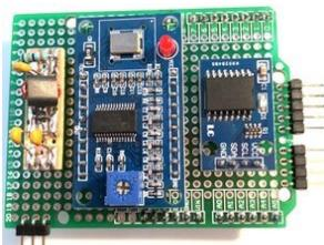
The Arduino shield with Buffer amp, Synthesiser and Real Time Clock.
