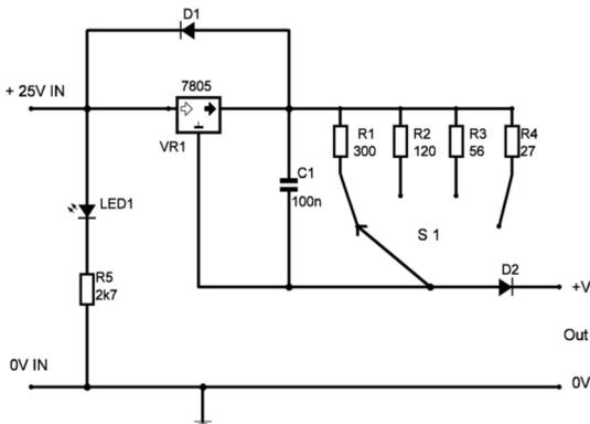
My aim was to have current output ranged in a binary sequence of 25 mA, 50 mA, 100mA and 200 mA with current set by a four-way rotary switch.
