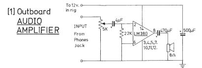
The above Outboard Audio Amp for the HW8 (or HW7) works very well and requires no hole to be cut in the rig. It is built into the speaker box with three leads going to the HW8 - input and 12- to the phones jack and 12+ an inline socket through one of the spare holes in the supply point. One could also fit a stereo socket to the rig to provide all 3 points
