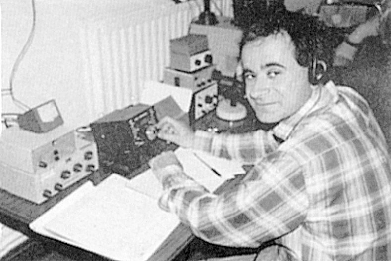
Bob Ross WA2MFI Operates EI3RJV During the International QRP Week in Dublin A QRP PLUS running into an experimental Memory ATU from Hands Electronics (above the TenTec Tuner)
