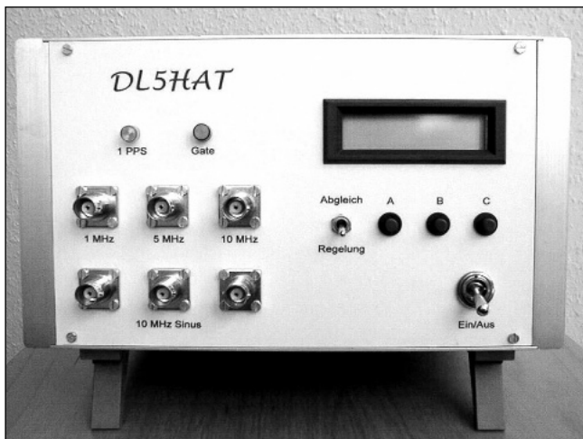
Fig 11.26: Picture of the prototype high precision frequency standard for 10MHz controlled by GPS
